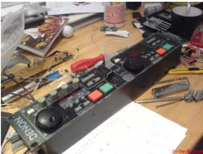
Position of future encoders for FX section.
