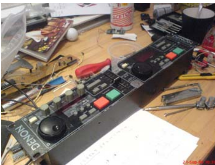
Position of future encoders for FX section.
