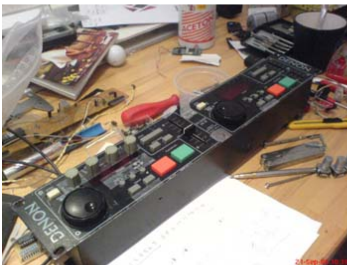
Position of future encoders for FX section.
